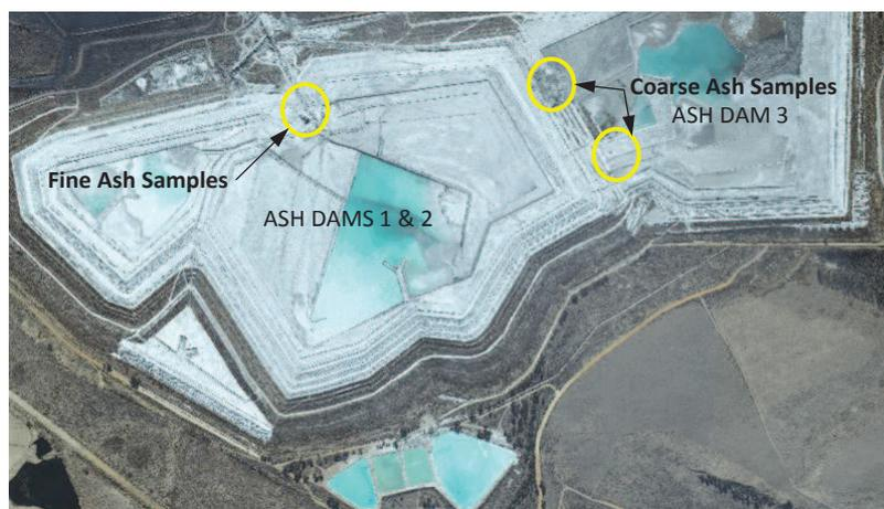
Figure 2-5: Ash Sampling Positions
